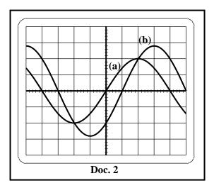
The oscilloscope, conveniently connected, allows us to display the voltage  $u_{AM}$  on channel ( $Y_1$ ) and the voltage  $u_{BM}$  on channel ( $Y_2$ ). The obtained waveforms are represented in document 4.
