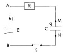
b- Knowing that the solution of this equation has the form:  $u_{C} = A(1 - e^{-\tau})$  determine A and  $\tau$ .
